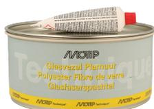
Universal two-component polyester putty to level irregularities in surfaces of steel, aluminium, wood, concrete and polyester. Polyester putty is elastic and very easy to sand. Polyester putty is re-sprayable with all lacquer systems and resistant to chemicals and the weather. Polyester putty can be applied in layers with a thickness up to 2 cm.
